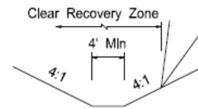
Preferred Trapezoidal Channel Section If Within CRZ
